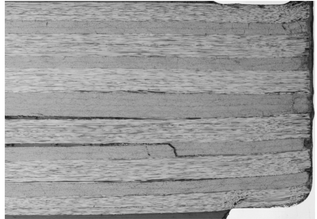
Fig. 21 Detail of the specimen struck with 50 kA, polished parallel to the 0 deg fibers in the proximity of the fastener head.
